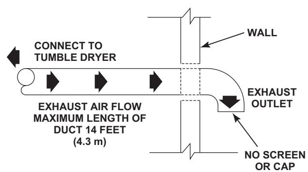
NOTE: WHERE THE EXHAUST DUCT PIERCES A COMBUSTIBLE WALL OR CEILING, AN OPENING HAVING A DIAMETER FOUR INCHES (10.2 cm) LARGER THAN THE DIAMETER OF THE EXHAUST DUCT SHALL BE PROVIDED AND THE EXHAUST DUCT CENTERED WITHIN THE OPENING.
